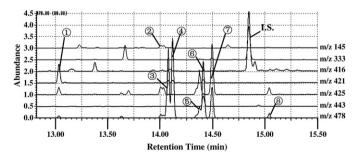
**Fig. 2.** Representative mass chromatograms of CBD metabolites formed by HLMs. Pooled HLMs (40 µg protein/ml) were incubated with 6.4 µM CBD for 20 min. The data, retention times, and typical fragment ions of CBD metabolites were listed along with their matching peak number in Table 1.
