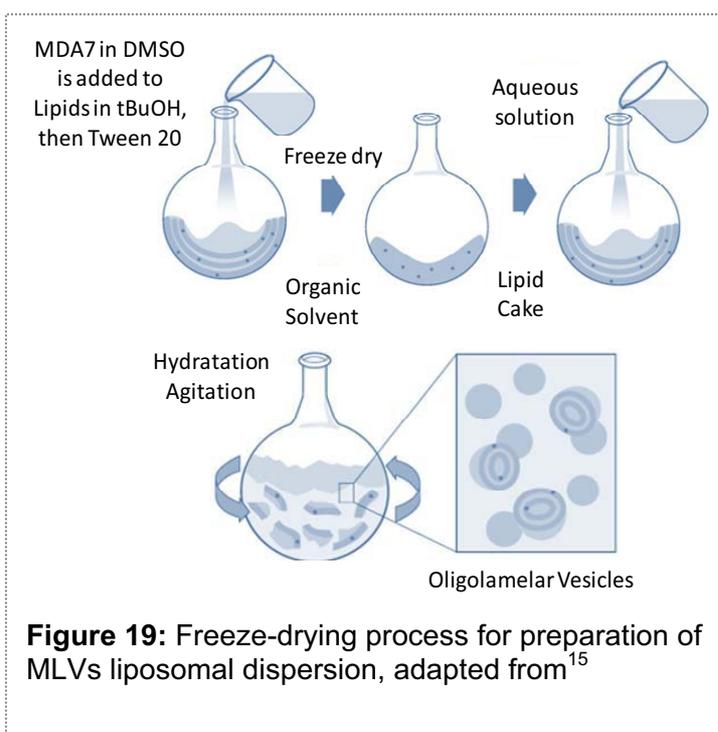
**Figure 19:** Freeze-drying process for preparation of MLVs liposomal dispersion, adapted from<sup>15</sup>
