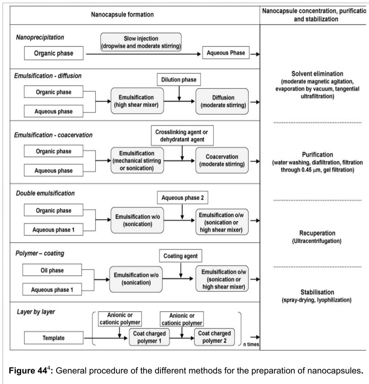
Figure 44<sup>4</sup>: General procedure of the different methods for the preparation of nanocapsules.
