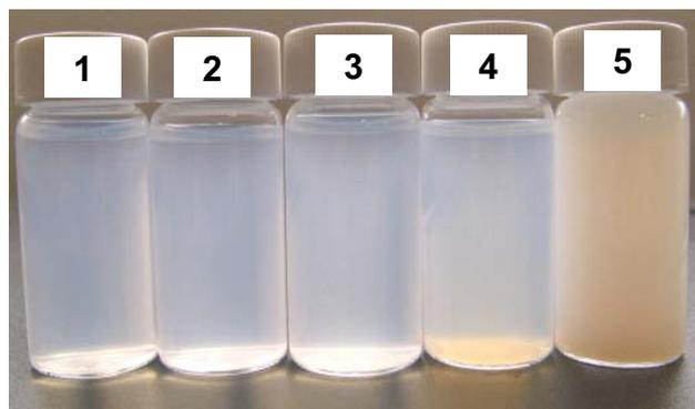
**Figure 56:** Picture of nanosuspensions prepared with increasing amount of polymer from left to right. 1, 2, 3, 4, are colloidal dispersions of polymeric NCs (Tyndall effect). 5, is opaque and composed of larger particles.
