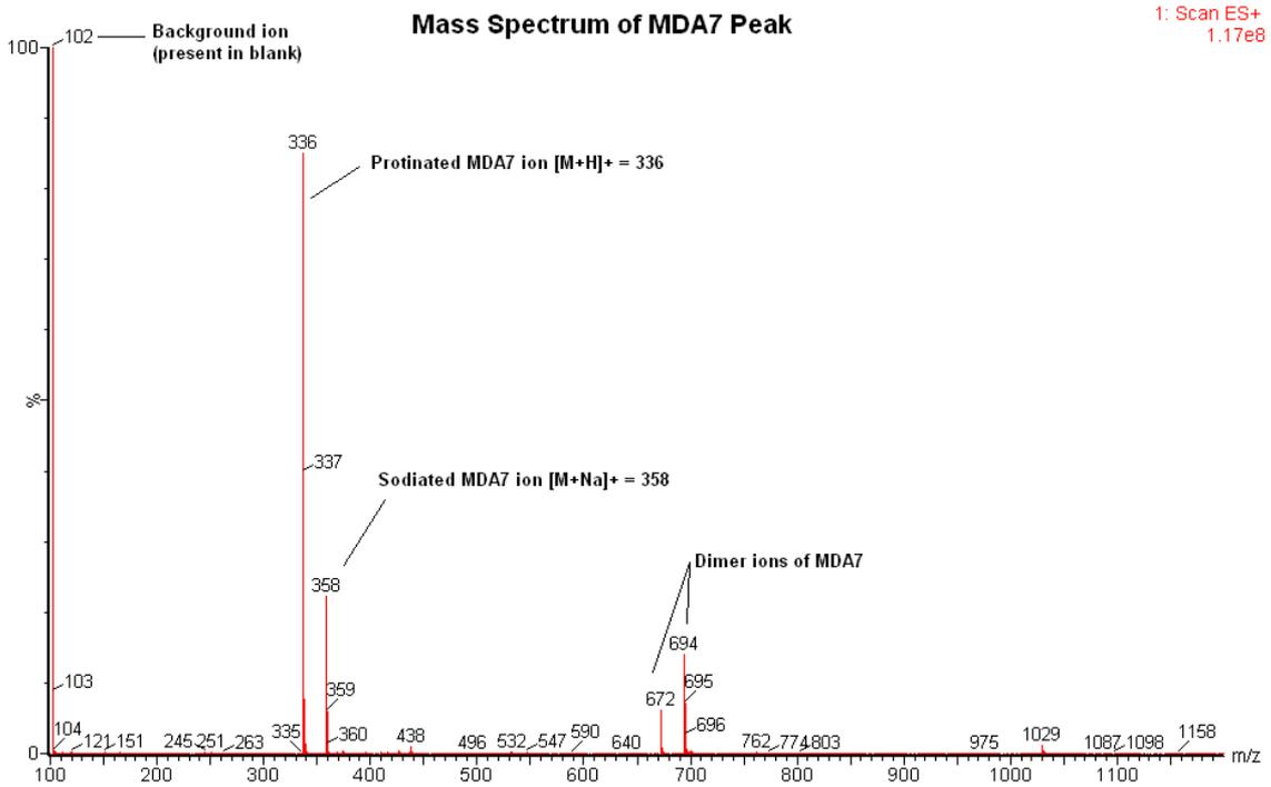
Figure 73: Mass spectrum of MDA7 peak in above MS chromatogram.
