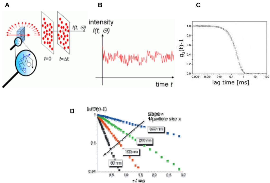
**Figure 18:** DLS measurement principle<sup>13</sup>.
