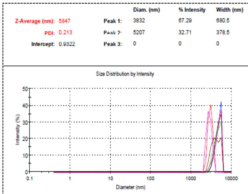
**Figure 107:** Particle Size distribution of entry 24 Table 37.
