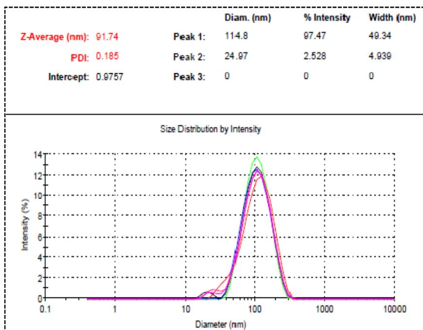
**Figure 106:** Particle Size distribution of entry 23 Table 37.
