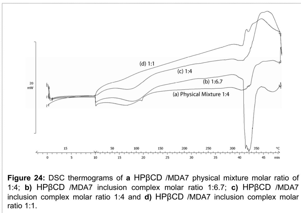
**Figure 24:** DSC thermograms of **a** HP $\beta$ CD /MDA7 physical mixture molar ratio of 1:4; **b**) HP $\beta$ CD /MDA7 inclusion complex molar ratio 1:6.7; **c**) HP $\beta$ CD /MDA7 inclusion complex molar ratio 1:4 and **d**) HP $\beta$ CD /MDA7 inclusion complex molar ratio 1:1.
